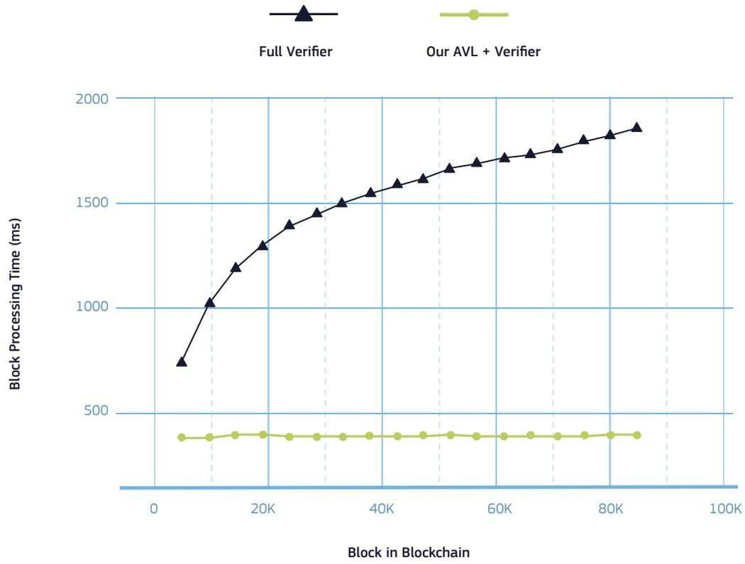
Fig. 14. Block processing time on blocks in blockchain dependency
